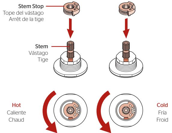
**Stem Stop can be inserted into Stem in either of two ways, depending on the rotation you want to have for your handles.**
