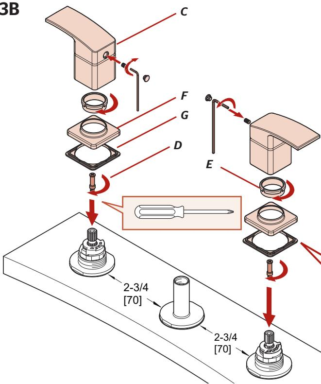
Apply Plumber's Putty in highlighted grooves beneath B and G (x2). If installing on marble, no putty needed.
